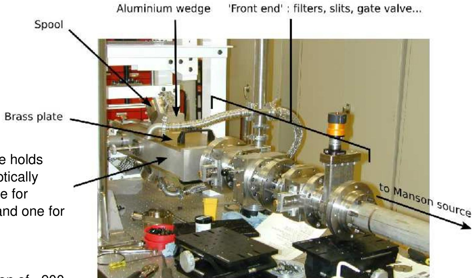
Crystal enclosure holds **two** identical elliptically bent crystals: one for **time integrated** and one for **time resolved** measurements
